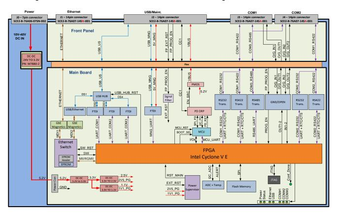
The MILTECH 2022 Unit is based on Intel FPGA firmware used for encapsulating and decapsulating the 3x UART ports over the Giga-bit Ethernet interface.
